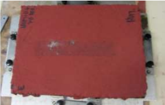
FIGURE 5- SLAB E AFTER 10 000 CYCLES
