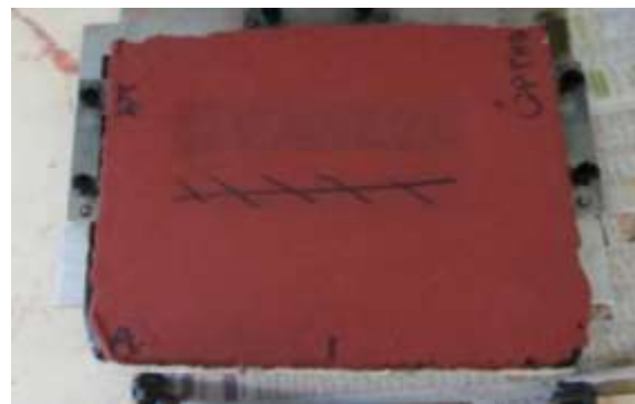
FIGURE 4 - SLAB D AFTER 10 000 CYCLES
