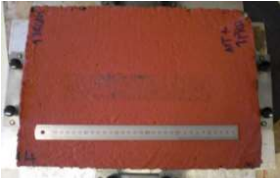
FIGURE 6- SLAB F AFTER 10 000 CYCLES
